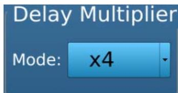
Use the drop-down button to select the Delay mode. Multiplies print delay between messages.
