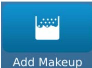
Will add a small amount of make-up to the reservoir. Performing this function will slightly lower viscosity.
