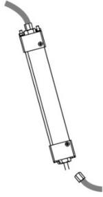
Disconnect the bottom tube of Viscosimeter
