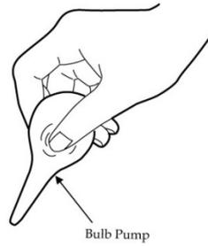
Use a bulb pump to absorb some solvent or cleaning solution
