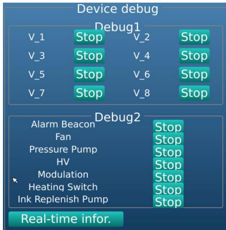
Device test window is only available if the hydraulics (jet) are shut down/off. A/C power must be on.
