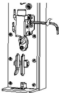
1. Loosen fixing screw.
