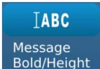
Increasing or decreasing the Height will raise or lower the text height. 100 is the maximum height. Setting Height too low may cause ink build-up on the gutter tube and affect print quality.
