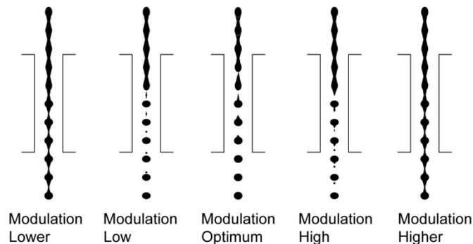
Before adjust the ink break-off position, make sure that the current ink viscosity is suitable for printing. Then find the magnifier to observe the ink break-off position in the charge electrode, adjust the modulation (Nozzle drive) to adjust the ink break-off position.
