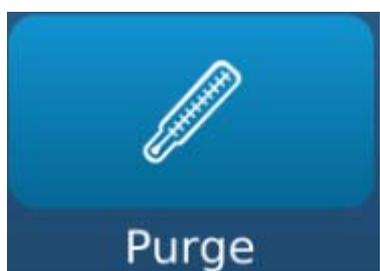
Selecting "Purge" will cause a light suction for about 20 seconds at the nozzle face. This is used when spraying cleaner externally onto the nozzle so the cleaning fluid can be drawn back into the Gunbody.
