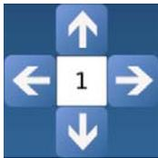
Click this button to move the selected field. The number in the middle of the button is the distance that move one time, which can be modified when large-span adjustment is needed. The maximum value can be set to 140.
