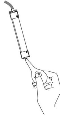
Press the bulb pump to clean the viscosimeter.
